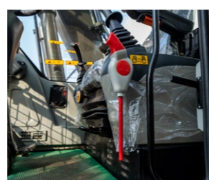
液压安全锁 Hydraulic safety lock
